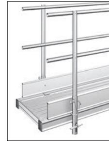
Assembly with **guardrail fixing** and **double guardrail with toe board**.
