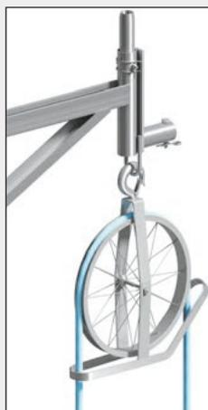
**Bracket 12** with **hoist wheel 13** for manual vertical transport of scaffolding material weighing up to 50 kg. Loads additionally applied to the scaffolding must be transmitted into the structure or into the ground by special measures, and additional anchoring may be necessary.
