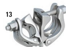
For connection at any angle of a tube dia. 33.7 mm to a tube of dia. 48.3 mm
