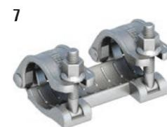
For connection of two tubes with dia. 48.3 mm in one axis. Only in conjunction with internal spigot Pos. 8
