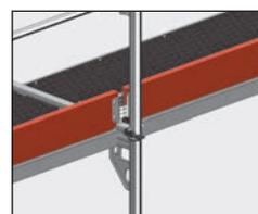
By using the **scaffolding lock**, you can secure your scaffolding against unauthorized alteration or dismantling. Use in topmost level instead of locking pins.
