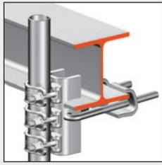
The **suspended scaffolding coupler 1** is suspended in existing brackets and I or U sections. With the three riveted-on half-couplers (for 48.3 mm scaffolding tubes) they have a permissible load of 15 kN.
