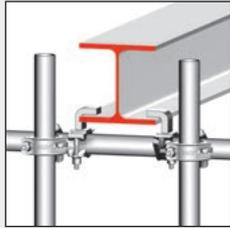
The **clamp couplers 3** for 48.3 mm scaffolding tubes are particularly advantageous for large flange widths. The connection to the flange is always made using two clamping couplers. Permissible load 9 kN per clamping coupler
