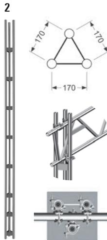
View onto lattice beam in triangular support, lattice beam is connected by swivel couplers to the support
