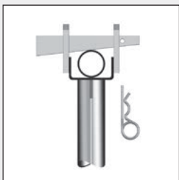
Detail for roof support
